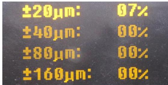
Press Up/Down to change the row. Select the desired range to calibrate. Press Left/Right to adjust the setting, then press Return to confirm the change.
