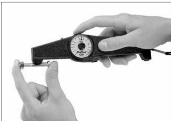
**Note:** *PosiTector* is available in two measuring ranges and in mils or microns scale.
