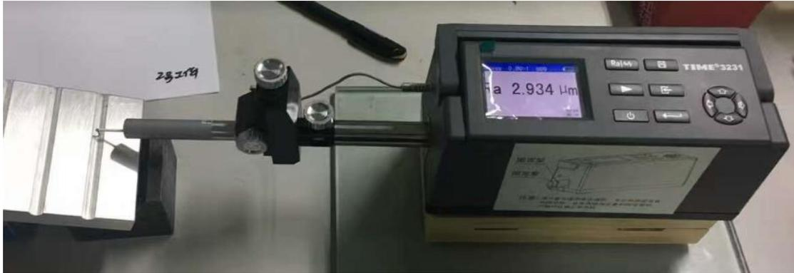
**90 ° Measurement with TIME3231 surface roughness tester**
