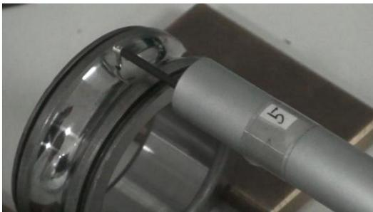
**External Raceway Measurement**
