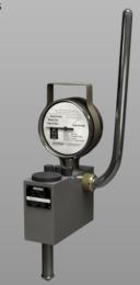
Long ram test heads are used with the 134 frame for testing over flanges, lips etc.
