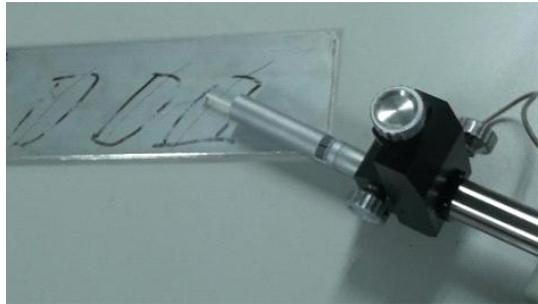
**Scratch Depth & Width Measurement**
