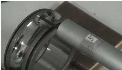
**External Raceway Measurement**
