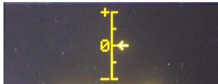
In main screen, press Return button to check the stylus position of the pickup. In general, for measuring in the plane, it is not necessary to adjust the position of the stylus. After measuring, the error of results is within the range of the instrument.
