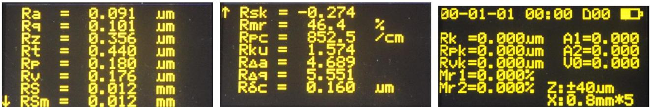
In the main screen, press Up to enter all Parameters Display screen. Press Up/Down to PageUp/Down. Press Set to return to the main screen.
