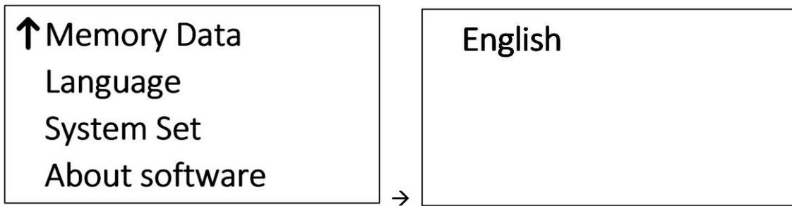
In main screen, press and hold Set to enter the main menu. Press Up/Down and select “Language”. Press Return to enter Language Select screen. Press Return to confirm and press Set button to exit.
