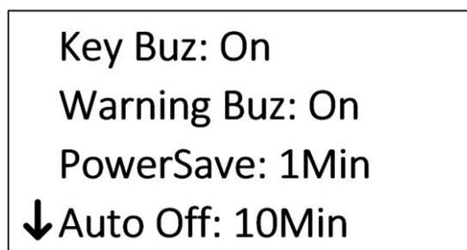
In the main screen, press and hold Set to enter Menu Setting mode. Select "System Set" to enter "System Set" menu item. Under this menu, you can set the following contents:
